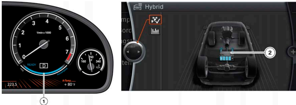
Displays for "Ready to drive" mode in the instrument cluster and CID
