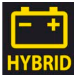
Check Control symbol for high-voltage battery
