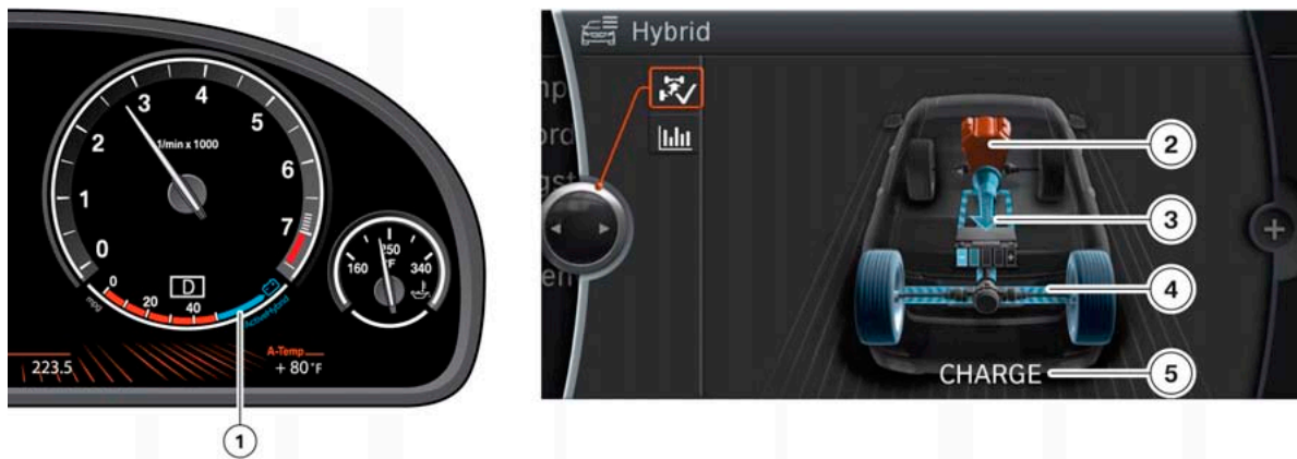
Hybrid displays in the instrument cluster and CID in overrun mode or when braking
