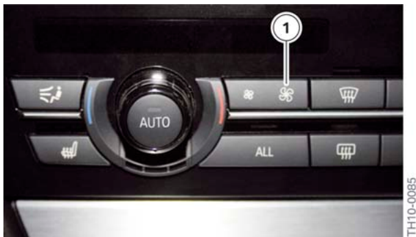
IHKA control panel
