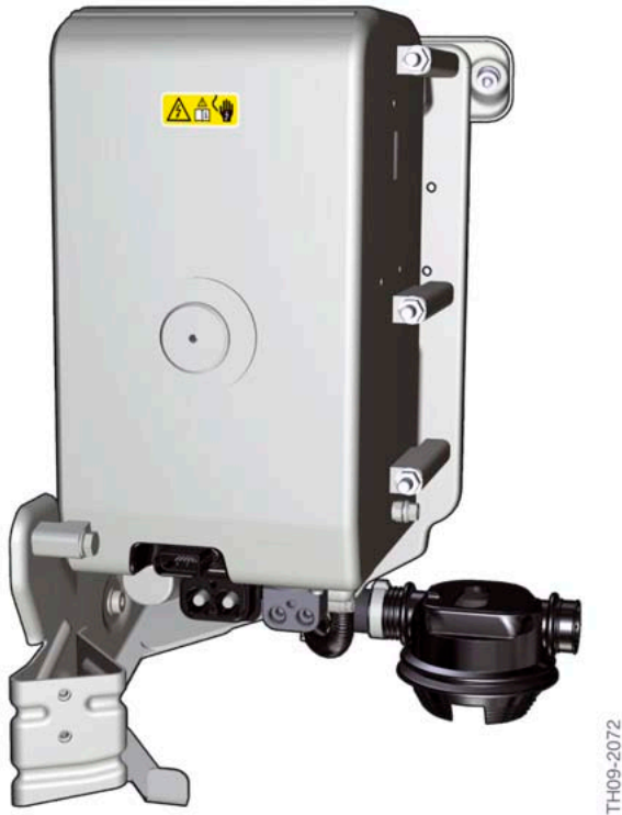
High-voltage battery in the F04
