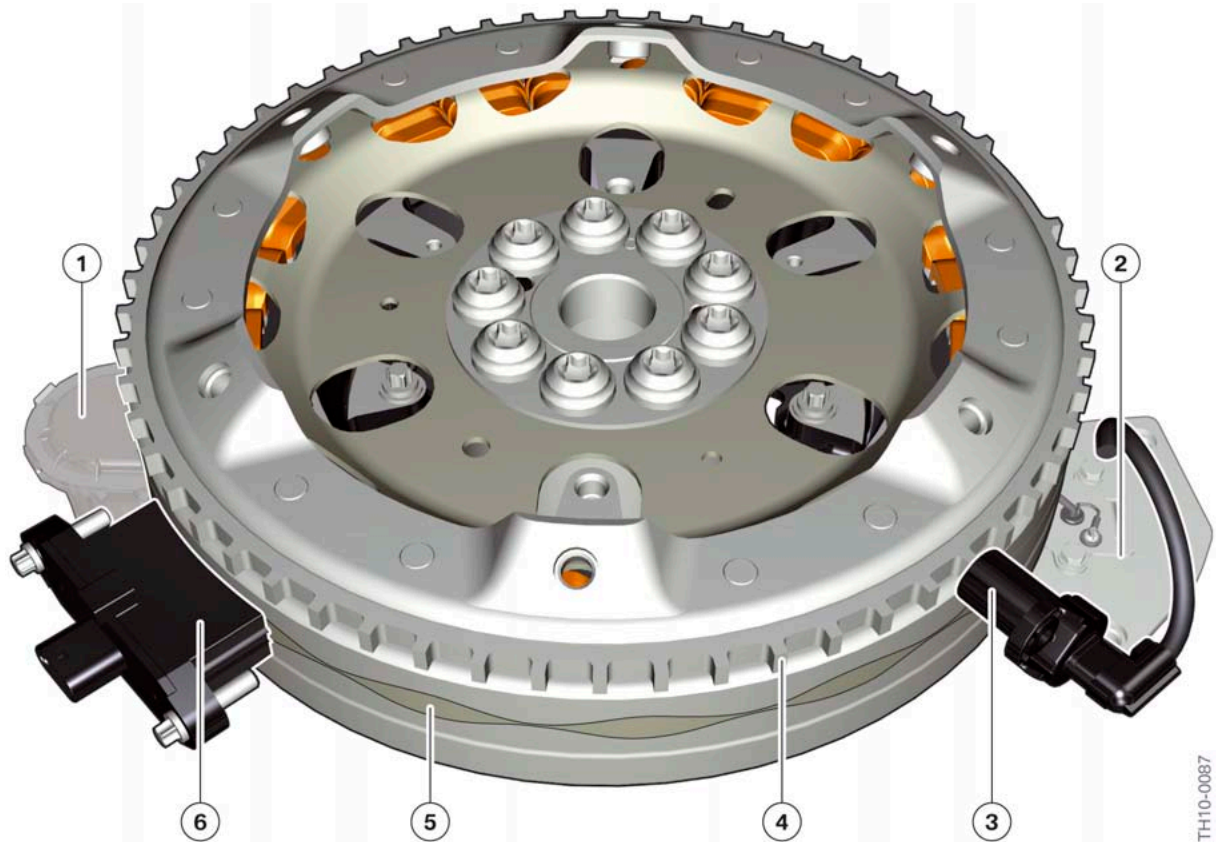
Sensors on the electric motor
